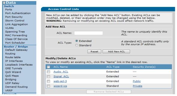
Start by creating an ACL which will be used to identify the SIP signaling traffic so that later on we can mark the packets with CS3.
